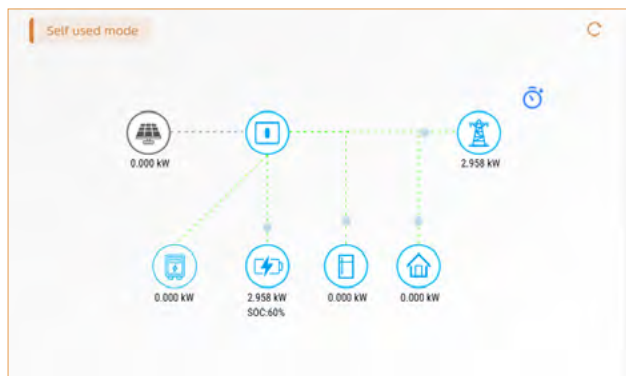
Figure 126. Generator web monitoring
